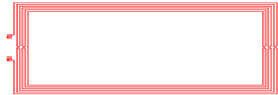
Figure 7. Reader antenna model of the rectangular antenna
