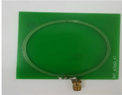
Figure 21. Built Prototype of the circular antenna
