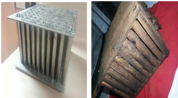
Figure 2. The photographs of the clean and fouled tubes.
