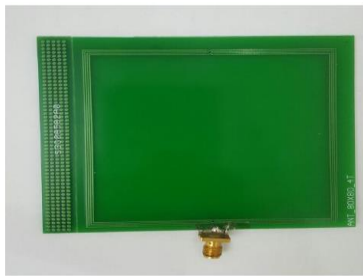
Figure 18. Built Prototype of the 4-loop square antenna
