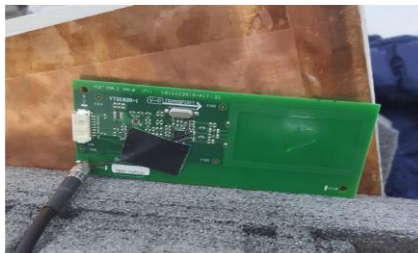
Figure 15. Metal effect with distance of 1 cm from the rectangular antenna
