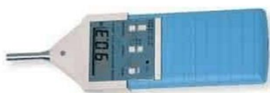
Figure 1. Sound measured meter (Model-CEL-231)
