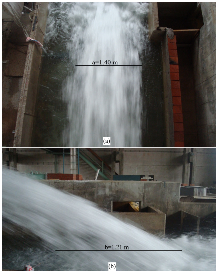
Figure 7 Lateral (a) and longitudinal (b) dimensions of the dispersed jet for Q = 0.22 \text{ m}^3/\text{s}
