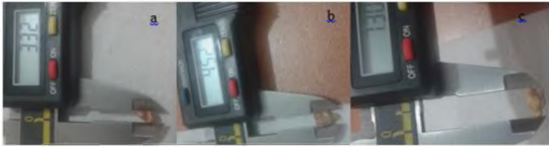
Figure 1. Method of measuring grape seeds a) method of measuring the thickness of the seed, b) method of measuring the width of the seed, c) method of measuring the length of the seed.
