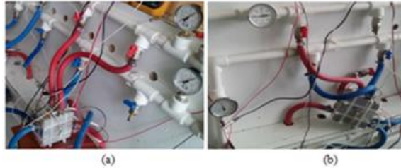
Figure 5. The image of sandwich blocks in the system with (a) hot-cold-hot (b) cold-hot-cold connection.
