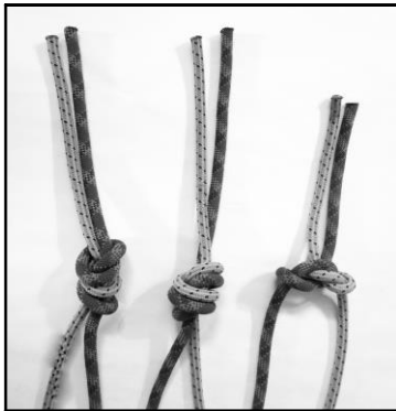
Figure 8. A sample of alternative side bends, which are more secure – Left to right: Figure Nine Side Bend, Double Overhand Side Bend, Alpine Butterfly Bend.
