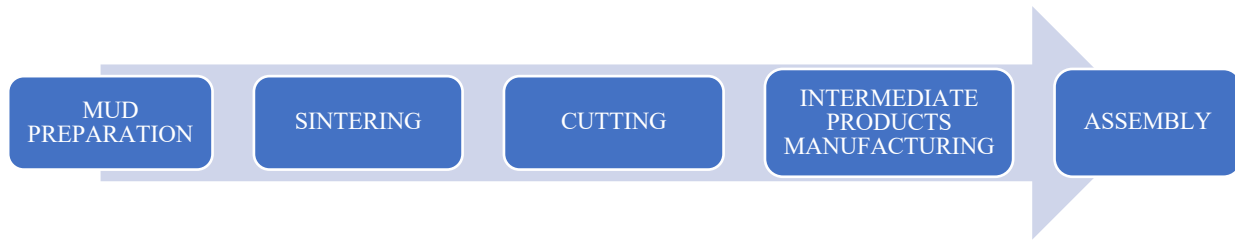
Figure 2. Medium voltage fuse production flow chart
