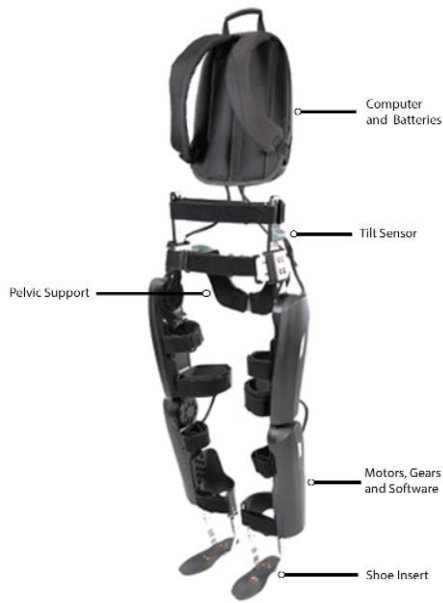
Figure 4. Sections of ReWalk LEE(Manns, Hurd, & Yang, 2019).
