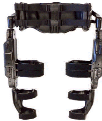
Figure 5. Vanderbilt Gait Assisting Exoskeleton.
