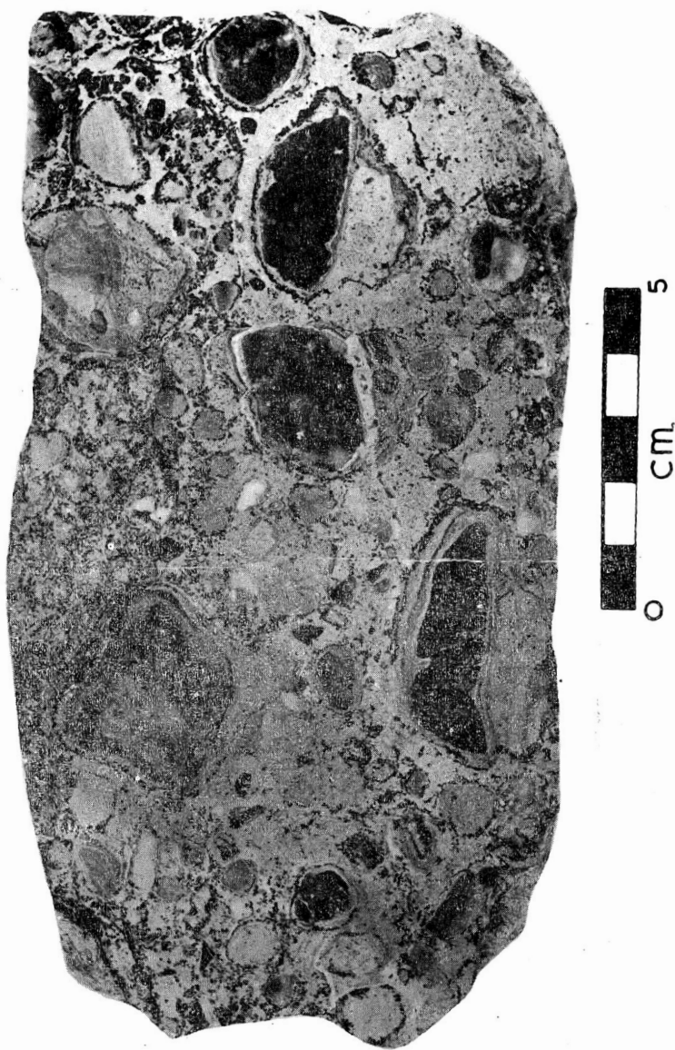
Plate: 1 — Hand specimen of the calcareous basal conglomerate (TL 212), showing concentrically arranged microcrystalline calcite around the pebbles.
