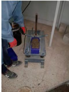
Figure 1. Vibrating Table
