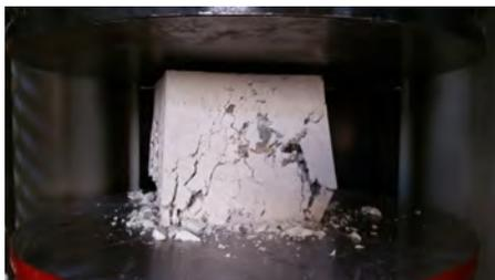
Figure 2. The compressive strength test (ASTM C39)
