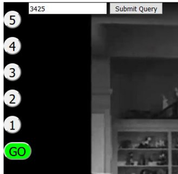
Figure 4. The proposed QoE evaluation interface compliant with the SSCQE method of ITU-Rec. 500-11.
