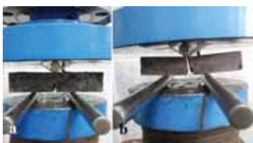
Figure 2. A three point flexural strength test specimen before loading (a) and after failure (b)
