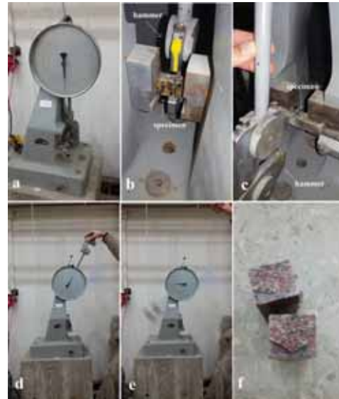
Figure 3. Charpy impact strength test: the test equipment (a), a specimen put in the abutments (b), lifting hammer (c, d), hammer dropped and determination of maximum hammer height after crack propagation (e), a failed specimen (f)
