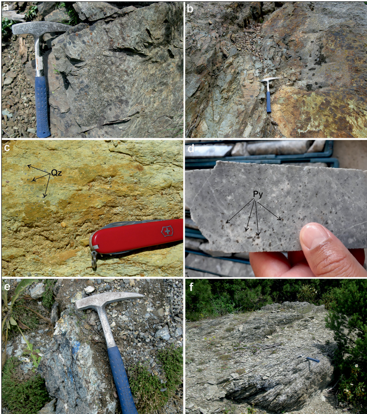
Figure 3- Field photographs of lithological units in the mineralization area. a) Metabasaltic andesite, b) limonitized altered metadacite, c) altered metadacite with semi-euhedral quartz minerals, d) aphanitic textured, silicified metariodacite containing disseminated pyrite, e) fractured zones containing azurite and malachite, f) phyllite (view direction north).
