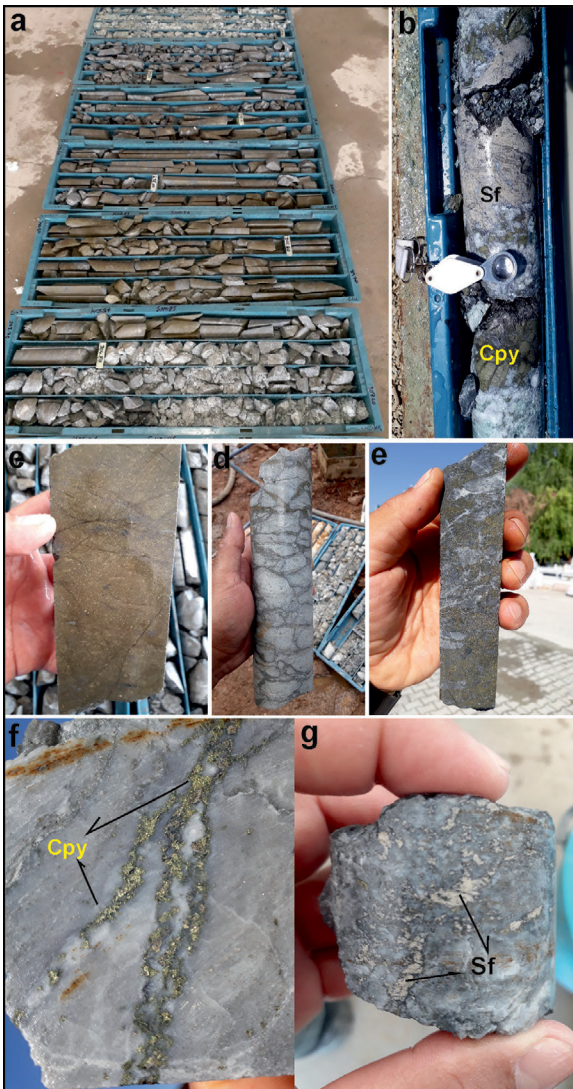
Figure 4- Core photographs associated with the Cünür mineralization. a) Massive sulfide ore with a thickness of 22 meters, consisting of massive ore, b) the appearance of zones rich in chalcopyrite and sphalerite minerals, c) the close view of the massive ore d) tectonic breccia fill secondary pyrite mineralization developed over silicified metariodacite, e) Substitution texture containing siliceous zones in semi-massive ores f) and g) appearance of chalcopyrite and sphalerite minerals filled with fractures and cracks in the silicified host rock.
