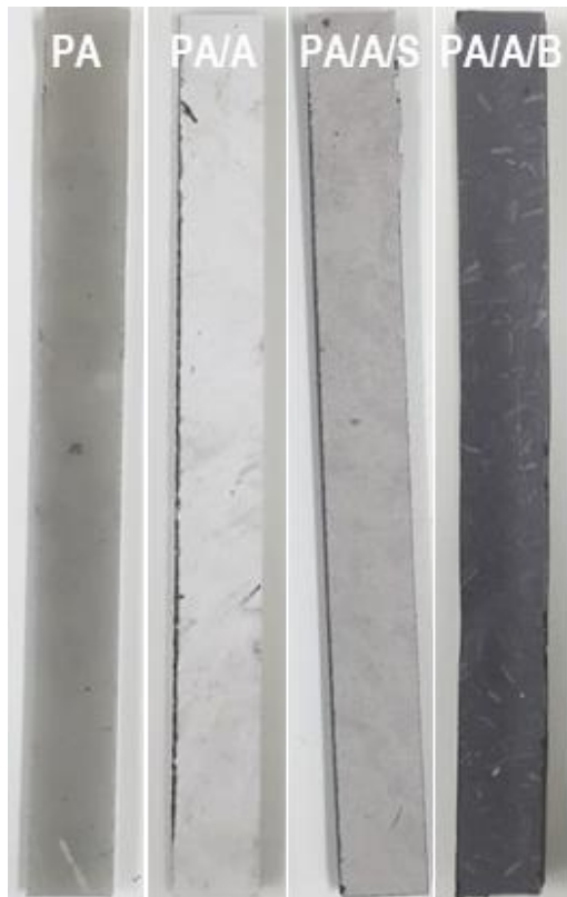
Figure 1. Images of prepared tensile and Charpy test samples
