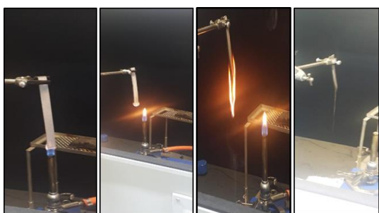
Figure 4. Images of composite materials during the vertical burning test
