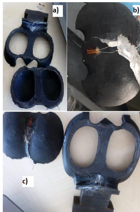
Figure 13. Breaking photos of a) Bucket #4, b) Bucket #5, c) Bucket #10
