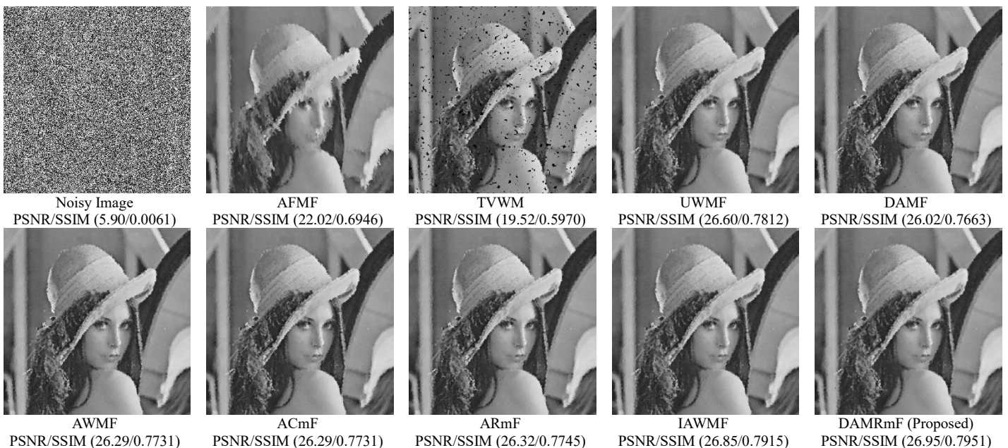
Figure 2. Image denoising results of the compared filters with SPN level of 90% of the "Lena" image (512 x 512 pixels).
