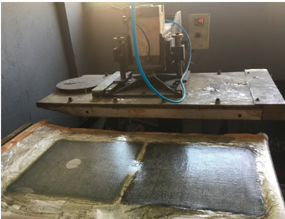
Fig. 1. Hot molding of composite plates.
