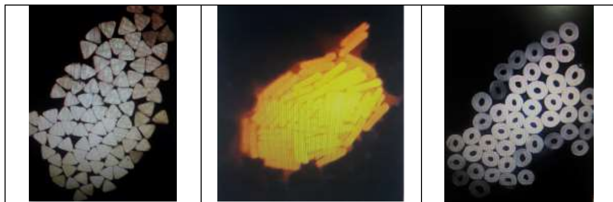
Figure 1. Cross-sectional view of produced polyester fibers: (a) trilobal, (b) flat, and (c) hollow captured with a magnification of 1000X
