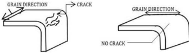
Figure 2. Example of Forming Error, Cracking [8]
