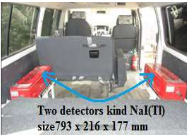
Figure 1. Two sodium iodide detectors NaI (Tl) inside the radiological survey field vehicle
