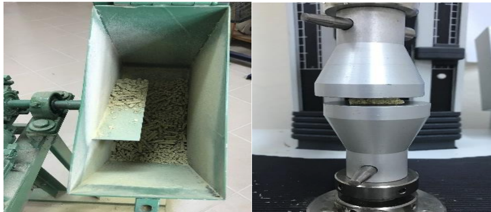
Figure 5. Mechanical durability and firmness tests Şekil 5. Mekanik dayanıklılık ve sertlik testleri
