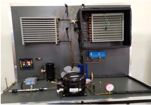
Figure 2. Experimental rig of refrigeration system
