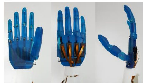
Figure 7. Images of the produced prosthetic hand in the open position
