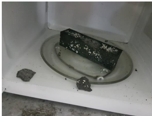
Figure 3. The effect of 300 W of MW curing on the sample after 30 minutes [14]
