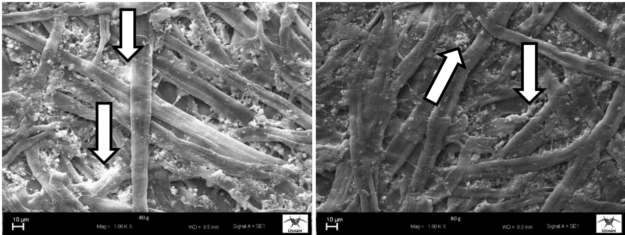
Figure 4. SEM images of recycled paper and base paper, Left: Base paper, Right: recycled paper
