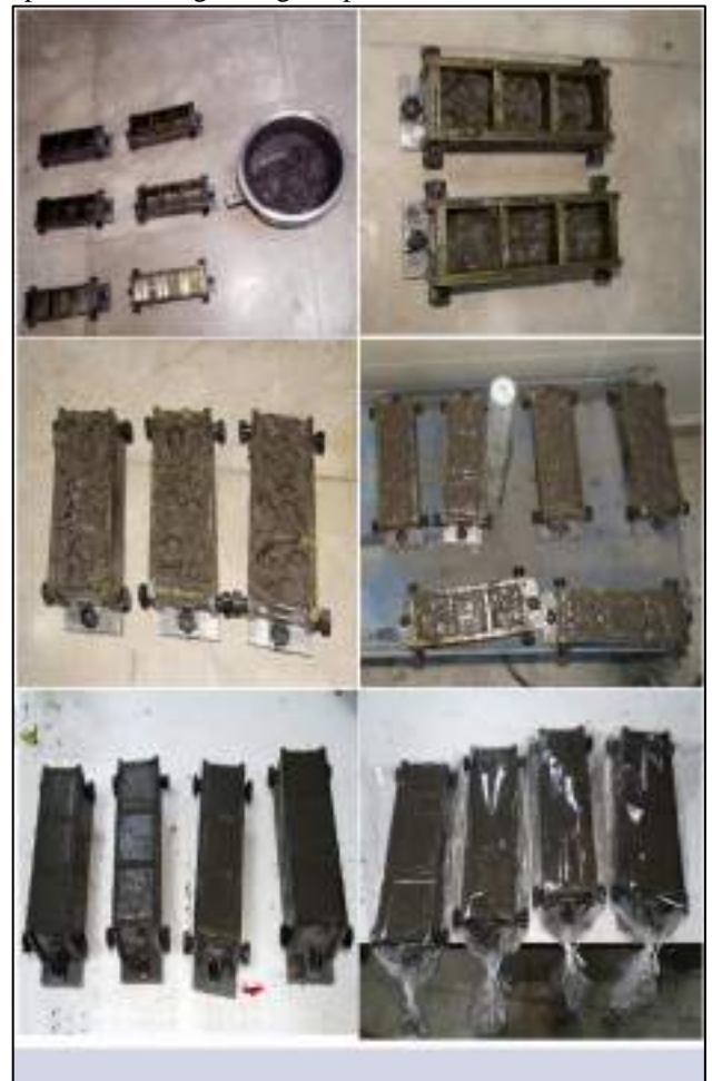
Figure 3 Casting geopolymer mortars
