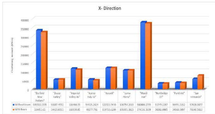
Figure 11. X- Direction Overturning Moment Values Comparison of the data obtained from both models
