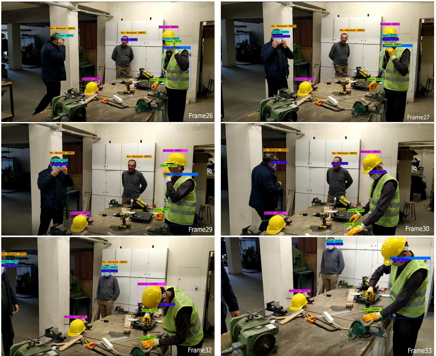
Figure 4. Object detection in the working environment on video frames using the proposed YOLOV4 model
