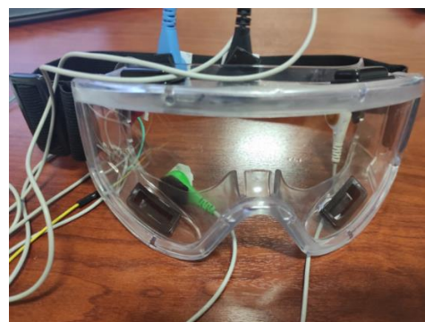
Figure 1: The glasses used for collecting EOG signals.
