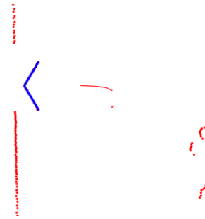
Figure 8 The model is executed again with a higher precision and accuracy, the goal point is set 0.5 meter in front of the reference point since in the docked state, the distance between the center of the robot and reference point is 50 centimeters.
