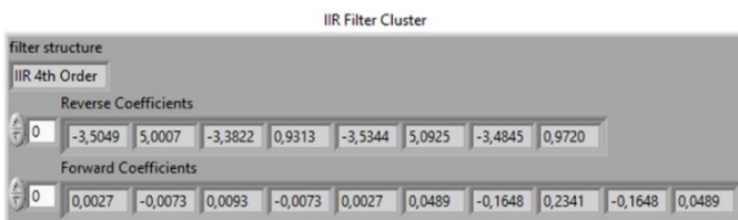
Figure 6. Filter coefficients of the elliptic IIR band-pass filter.
