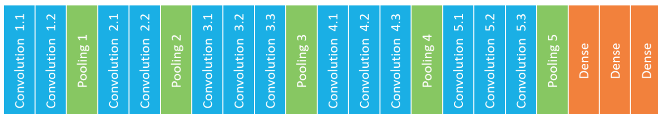
Figure 6. Structure of VGG-16 model
