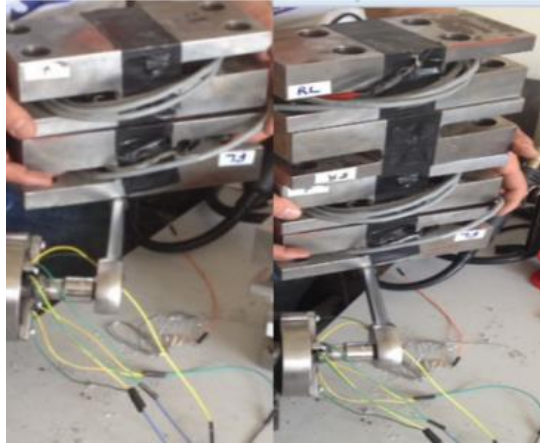
Figure 7. Application of 139.3 N and 278.6 N forces on the torque meter.
