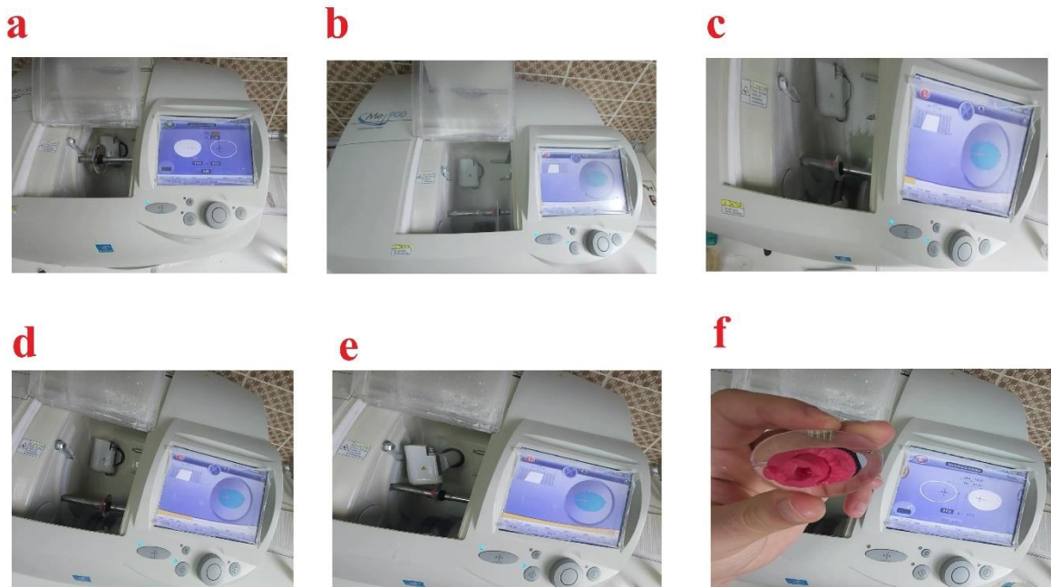
Figure 11. Figure illustrates lens placement (a), grinding (b), smoothing (c), polishing (d), edge cleaning (e) processes and the final product (f).
