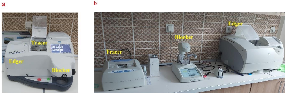
Figure 8. Figure illustrates edgers with internal tracer and blocker (a) and edger with external tracer and blocker (b).
