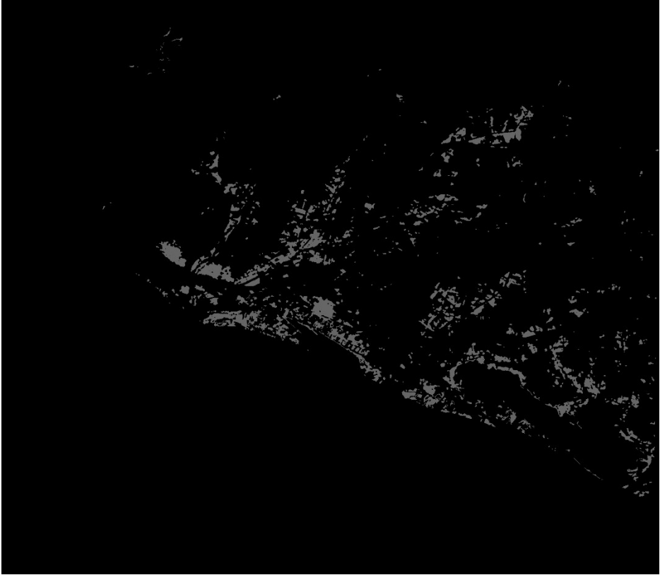
Figure 6. Sentinel 1 'after event' image composite after Otsu thresholding for VH polarization
