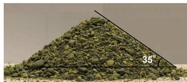
Figure 2. The angle of repose of the sand
