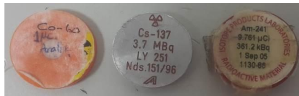
FIGURE 11. Radioactive sources ( ^{241}\text{Am} , ^{137}\text{Cs} , ^{60}\text{Co} ).
