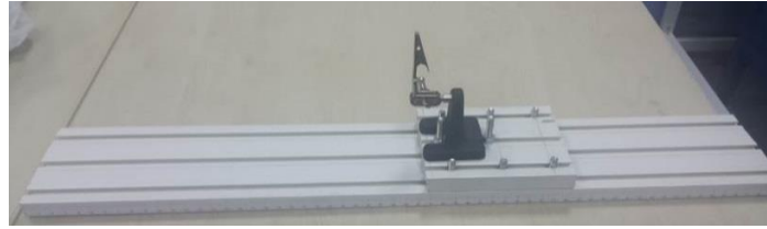
FIGURE 10. Source holder and sliding rail.
