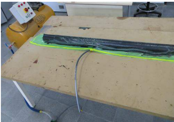
Figure 5 Vacuum process for CRP pipe after manufacture step.
