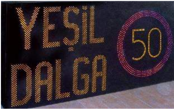
Figure 4. A VTS showing the speed limit indicating the green wave area.
