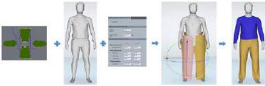
Figure 1. Process steps of 3D virtual garment simulation
