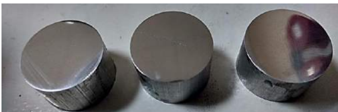
Figure 2. The mirror-like surface of the polished specimens
