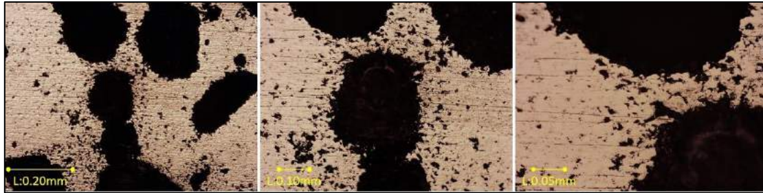
Figure 9. Optical microscopy of Ti/HA 50% porous scaffolds, \times 50 , \times 100 and \times 200 respectively
