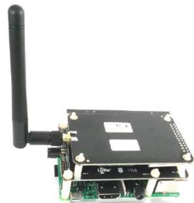
Figure 4. RAK831 based LoRa gateway with Raspberry Pi
