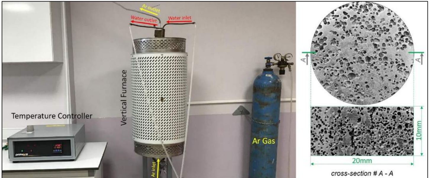
Figure 6. Final sintering trial setup; vertical furnace with Ar gases sweeping from bottom to top and successfully sintered scaffolds
