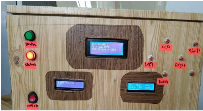
Figure 16. Supervision & control interface
