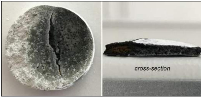
Figure 5. Scaffold which obtained with a second sintering trial with a cross-sectional image
