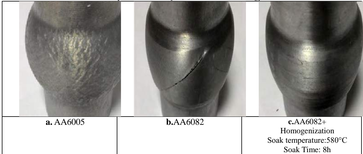
Fig 3. Macrostructure features of samples after cold forming process (a. AA6005, b. AA6082, c. AA6082+homogenization )
