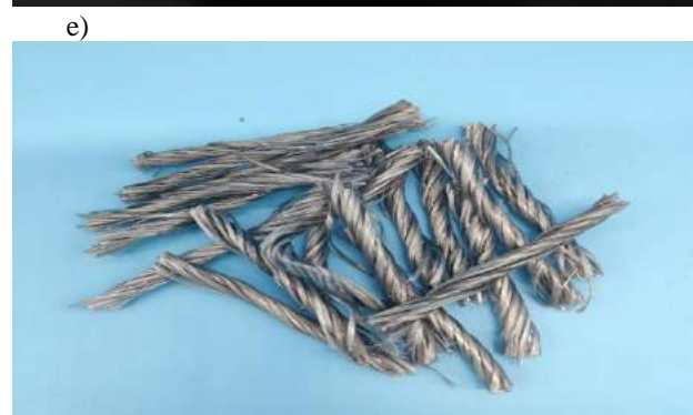
Fig. 3 Samples of a) steel-hook ended b) steel-crimped c) elastoplastic d) macro nylon e) macro twisted fibers
