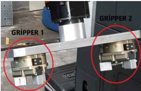
Fig. 1 The Standard Pneumatic Gripper Used as an End Effector in this Study.
