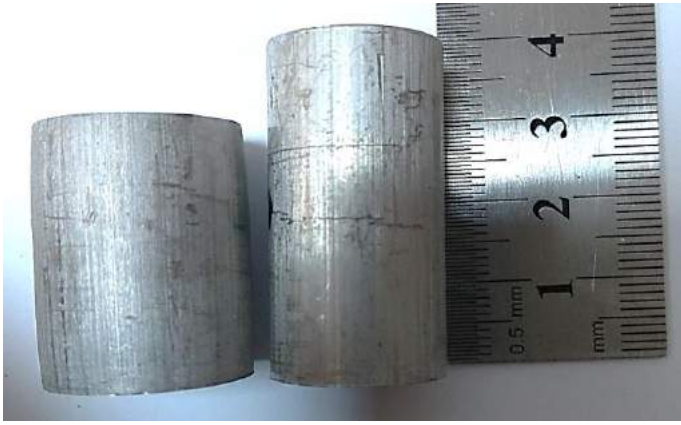
Figure 1. Specimens prepared from m AA6082 before compression test (right), after the test (left)
