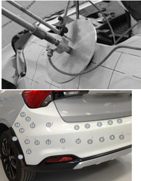
Figure 8. a) Typical physical test setup for denting resistance b) Loading point assessments
