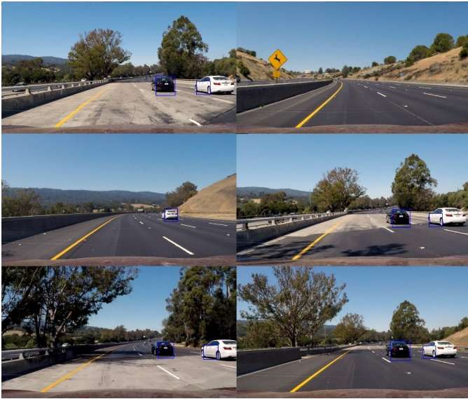
Figure 1. Vehicle detection in images with \text{hitThreshold}=1.25 and \text{finalThreshold}=0.75 with mean shift grouping
