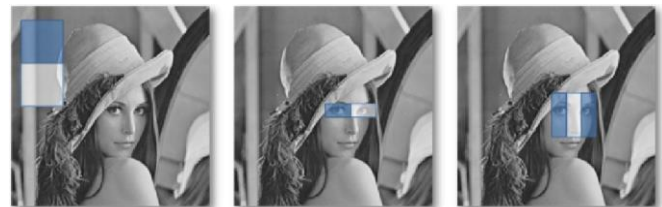
Fig. 1. The working principle of Haar-like features. Rapid face detection can be achieved by calculating features (the difference of the sum of pixels of white and blue rectangles)
