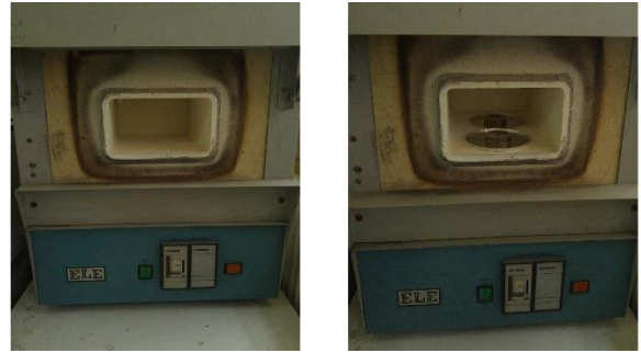
Figure 9 Resin consumption testing of filled composites
