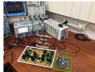
Figure 11 The built experimental laboratory set-up of the regulator system
