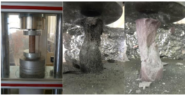
Figure 7 The pressure test of the filled composites
