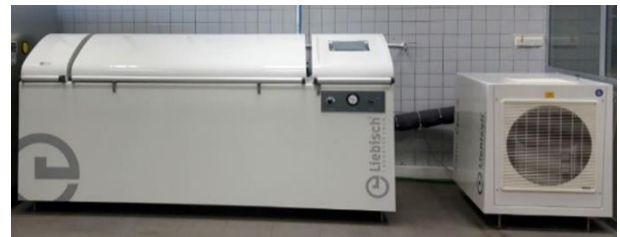
Figure 2 Test equipments; (a) Axial load fatigue and (b) salt spray testing chamber.
