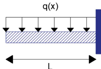
Fig. 1. A cantilever nanobeam which is uniformly loaded
