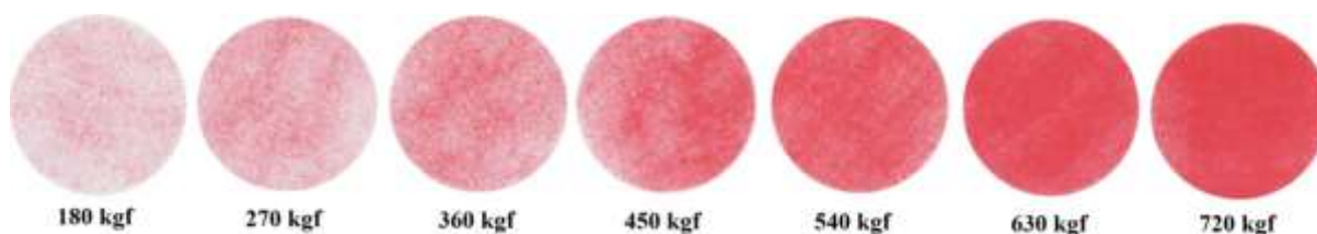
Figure 2. The red stains images of the samples subjected to different loads
