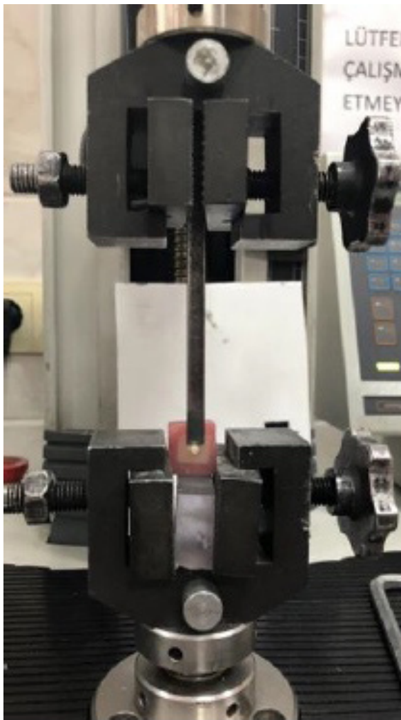
Figure 3. The specimen under the SBS test in the universal testing machine.
