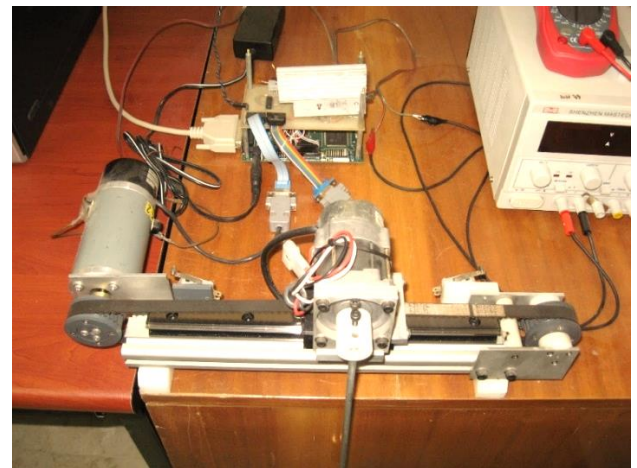
Figure 5. Hardware implementation of the inverted pendulum (Gün,A. 2007)
