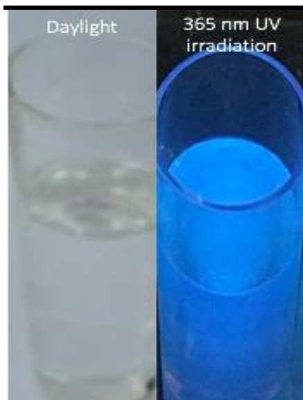
Figure 5. Daylight of Hypericum perforatum L. flower carbonized at 250 °C and UV irradiation image at 365 nm wavelength
