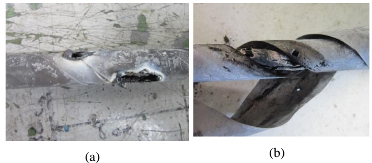
Figure 3 The Structural View of cable after test operations; a) 250V applied state, b) 500V applied state
