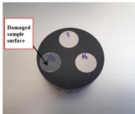
Figure 11. One of the 24 wt.% B 4 C reinforced samples where surface damages occur
