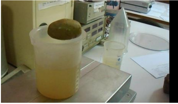
Figure 3. Measurement of volume of potato tuber by using water displacement method.
