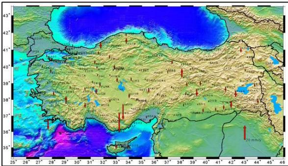
**Figure 6.** Point velocities (vertical) (Özdemir et al., 2011)
