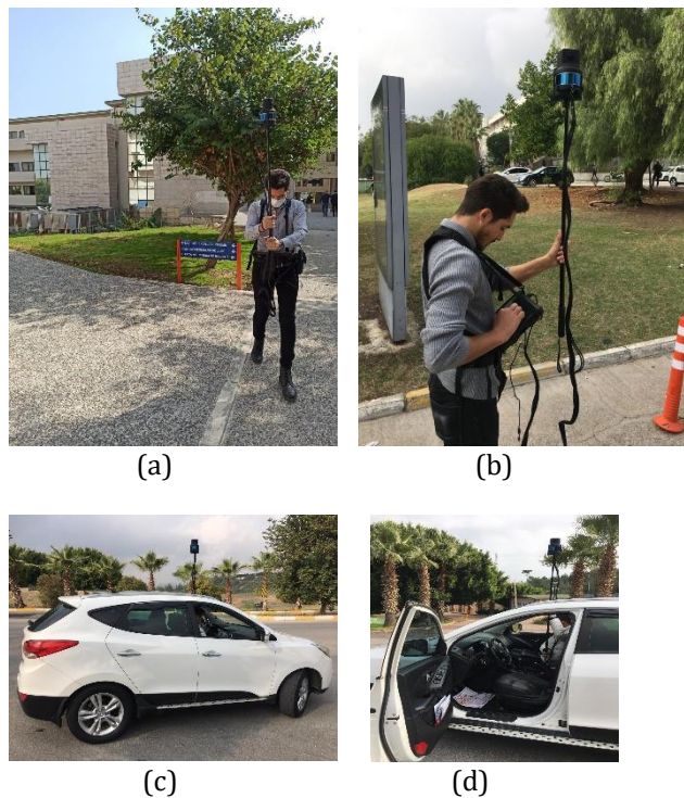
Figure 10. (a) and (b) Scanning with the wearable laser scanner (c) and (d) using the laser scanner device in the vehicle
