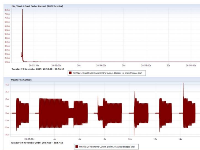
Figure 17. Change of inrush current and crest factor obtained for 2x36 W for fluorescent lamp with magnetic ballast
