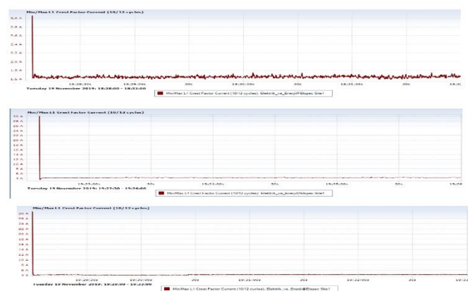
Figure 31. Graphs of crest factors of different LED loads (LED bulb at the top, LED panel in the middle, and LED projector at the bottom)
