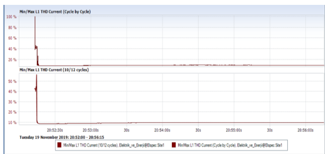
Figure 15. Change of THD (Total Harmonic Distortion) value of L 1 phase current during 32 W measurement
