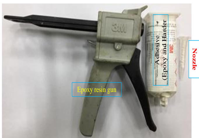
Figure 5. Equipment used in the bonding processing
