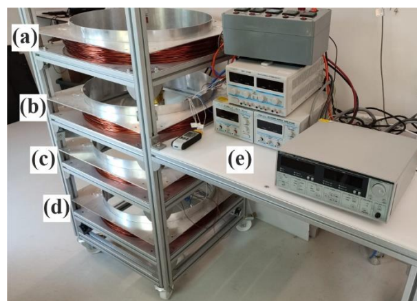
Figure 2. Constructed system: (a) I-element, (b) II-element, (c) III-element, (d) IV-element, and (e) power supplies.
