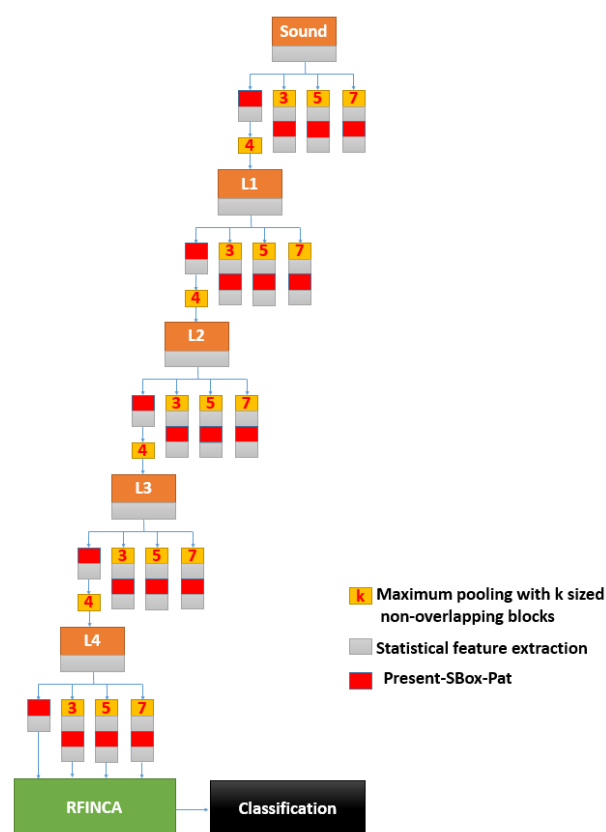
Figure 1. Graphical summarization of the proposed Present-SBox and RFINCA based breathing lung sounds classification method.
