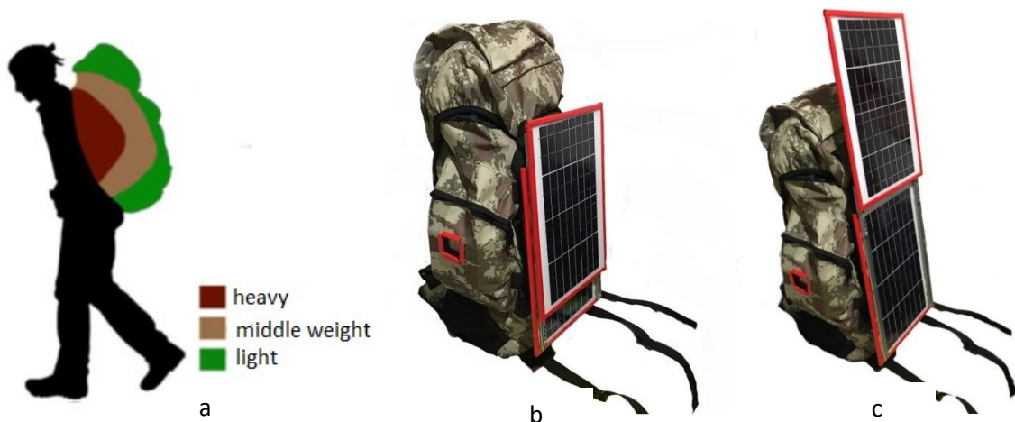
Figure 7. a) Distribution of weights on the backpack b) Prototype of the backpack (one solar panel active) c) Prototype of the backpack (two solar panels active)
