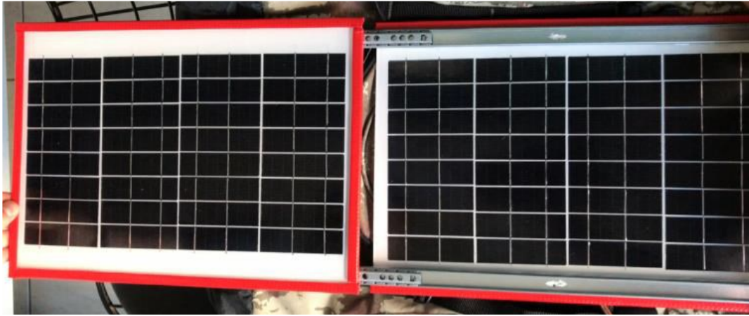
Figure 2. Double layer solar panel
