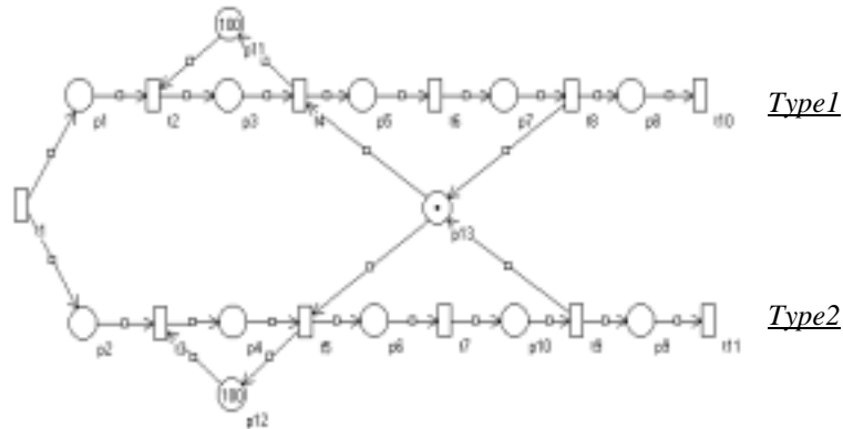
Figure 5. A Petri Net Model of One Machine-Two Product System
