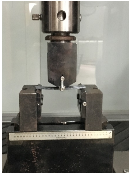
Figure 4. Application of three-point bending tests on CFRTP samples
