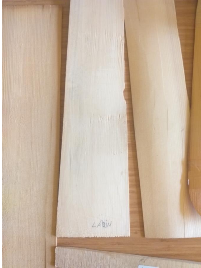
Figure 3. Spruce tree with annual rings close to each other and prepared for the cover of the high-pitched kemençe (Ceyhun Demir’s archive, 2019).
