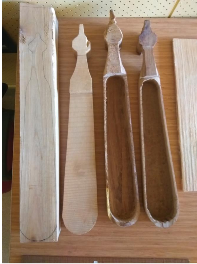
Figure 2. The process from templating the kemençe to carving the body (Ceyhun Demir's archive, 2019).
