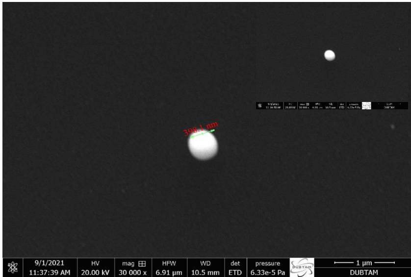
Figure 6. SEM image of Ag NP produced by PLD for 24 minutes (14400 laser pulses).
